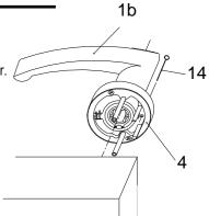
• On the other side insert the rose base plate (4) so that the female thread lines up with the male thread, and fasten with 1 1/4" (31.75mm) machine screws (3).
