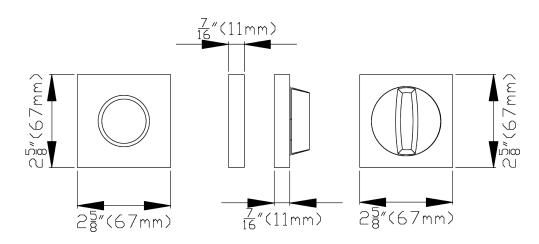
Please note: Karcher Design produts are designed and measured in metric. Imperial measurements are close approximations to the actual metric dimensions
